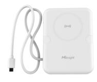
VS373 is a Radar Fall Detection Sensor<sup>1</sup> that adopts a Millimeter Wave Radar to capture falling. It provides non-contact person detection through point cloud data and realizes fall alarms. With a fall detection accuracy rate of up to 99%, it ensures the safety of users.
