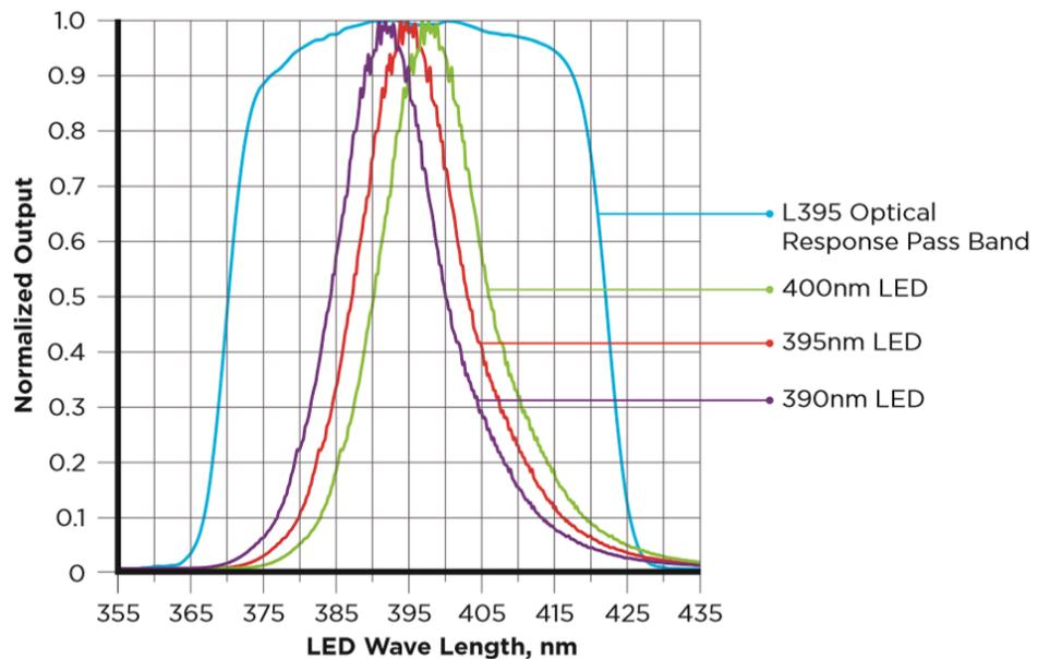
The Total Measured Optical Response (TMOR) for the EIT L-395 band shown above accurately captures all of the energy wavelengths emitted by a nominal 395 nm  $\pm$  5 nm LED (purple, red, green). The same is true for the response of all EIT L-Bands.
