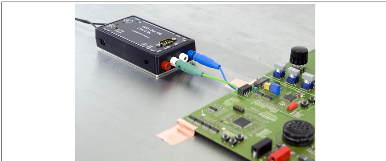
Figure 2: Opto-Box 100 in LIN mode, measurement set-up for measurement during development
