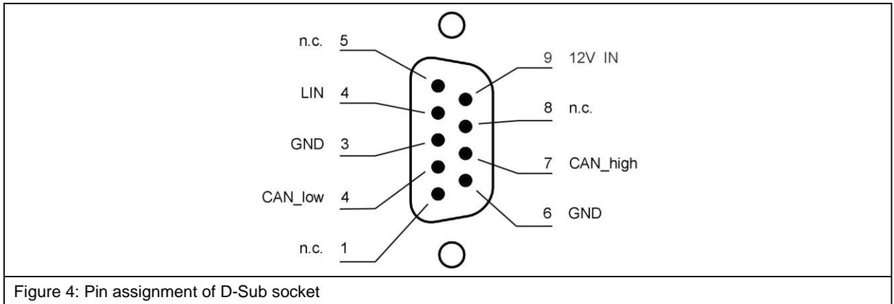
Figure 4: Pin assignment of D-Sub socket
