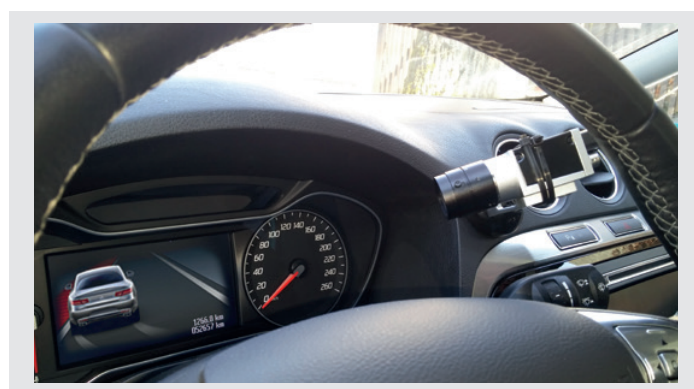
Picture Camera and microphone are mounted close to the combined instrument with a suction cup. There is no interaction during the trip.
