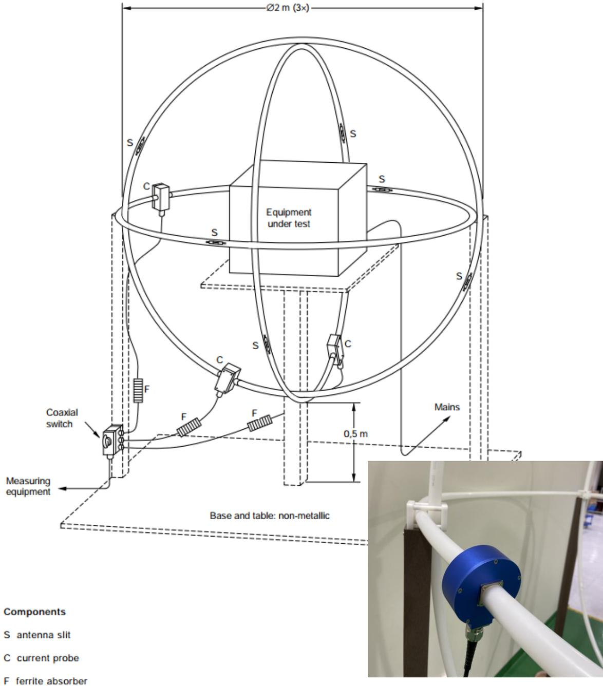
Figure 4: CISPR 16-1-4 / CISPR 15 large loop antenna
