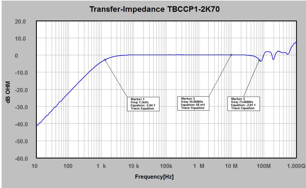
Figure1: transfer impedance, 10 Hz – 1 GHz, typical data
