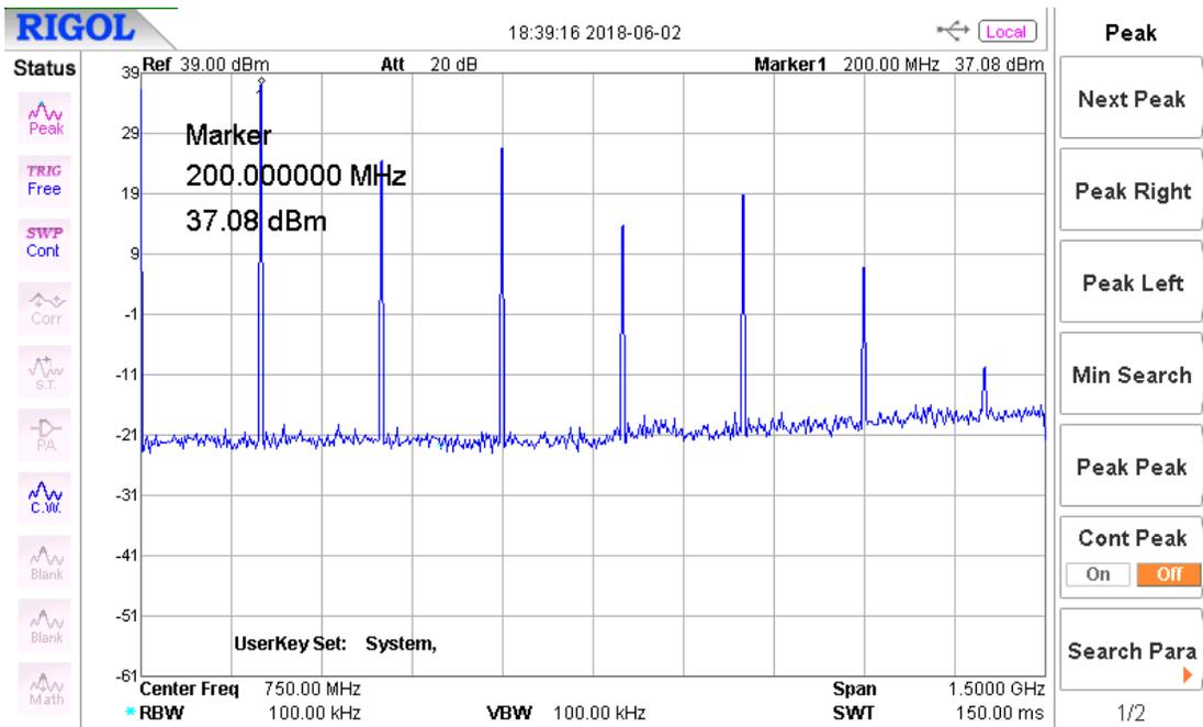
Figure 5 – CW, harmonics, 200 MHz
