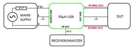
Figure 1 – Basic AC LISN set up: impedance levels
