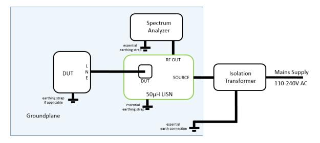
Figure 3 – Conducted noise pre-compliance measurement setup
