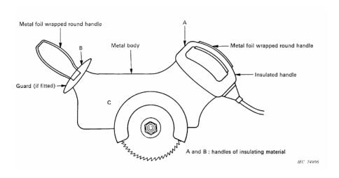
Figure 114 - Example from CISPR 16, portable electric saw with artificial hand
