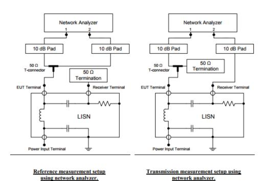
Figure 70 - Calibration set up according to CISPR 16-1-2 Annex A.8.
