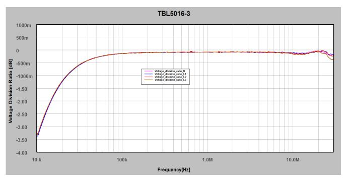
Figure 81 – Voltage Division Ratio versus frequency
