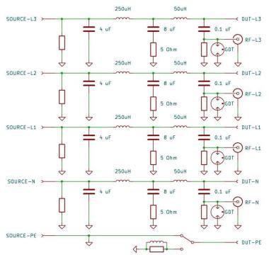
Figure 2 – 3-phase LISN, simplified schematic
