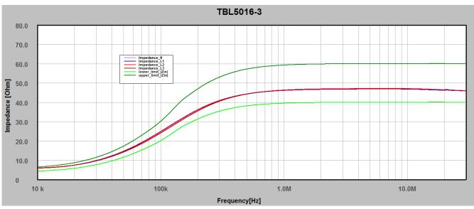
Figure 7 – Impedance vs. frequency at DUT terminals, limit lines according CISPR 16-1-2\*
