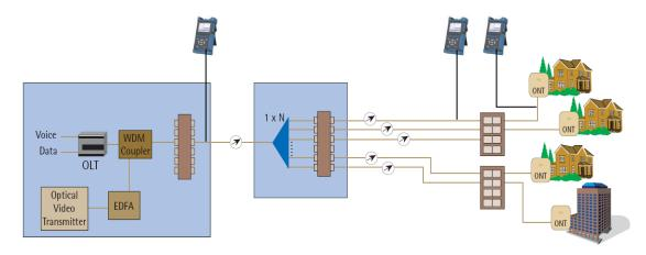
6416 Palm OTDR is mainly used to test FTTx network. It provides a low cost test solution for users. 6416 offers three test modes: manual (real-time, averaging), automatic, and dead zone.
