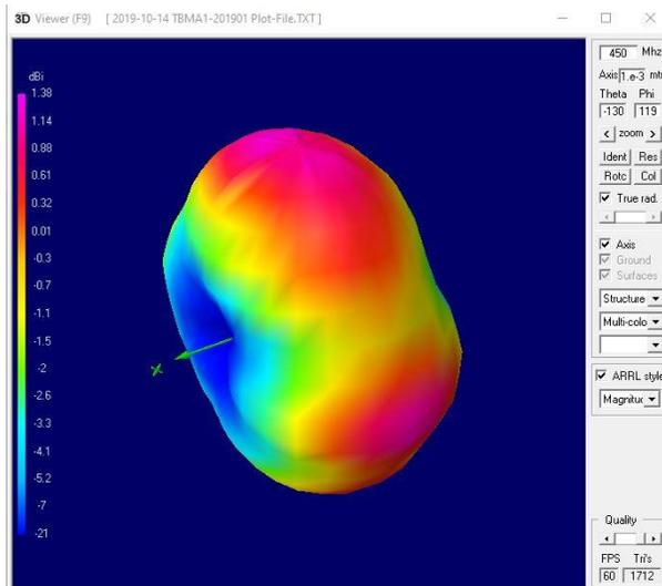
radiation pattern of the TBMA1 at 450 MHz
