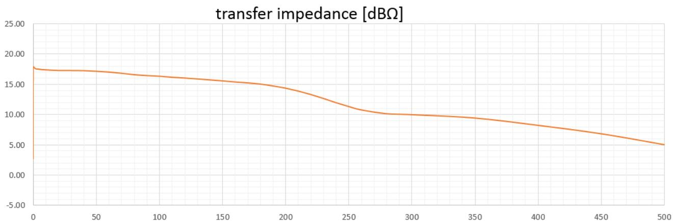
Figure1: Transfer impedance: 10 kHz to 500 MHz, linear
