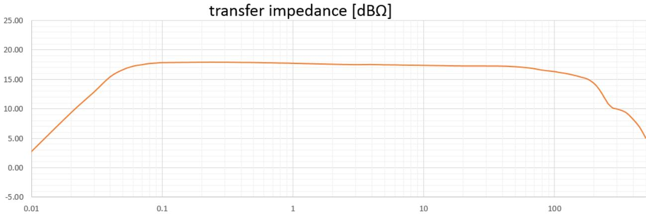
Figure2: Transfer impedance: 10 kHz to 500 MHz, logarithmic
