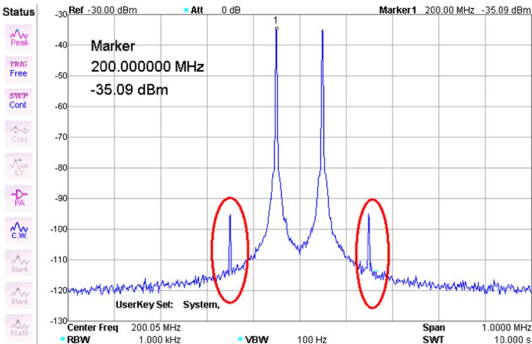
The following spectrum shows the spectrum of the same set up, however using the TBHDR1 pre-amplifier instead of the internal amplifier of the analyzer. Due to the high IP3 of the TBHDR1, the amplitude of
