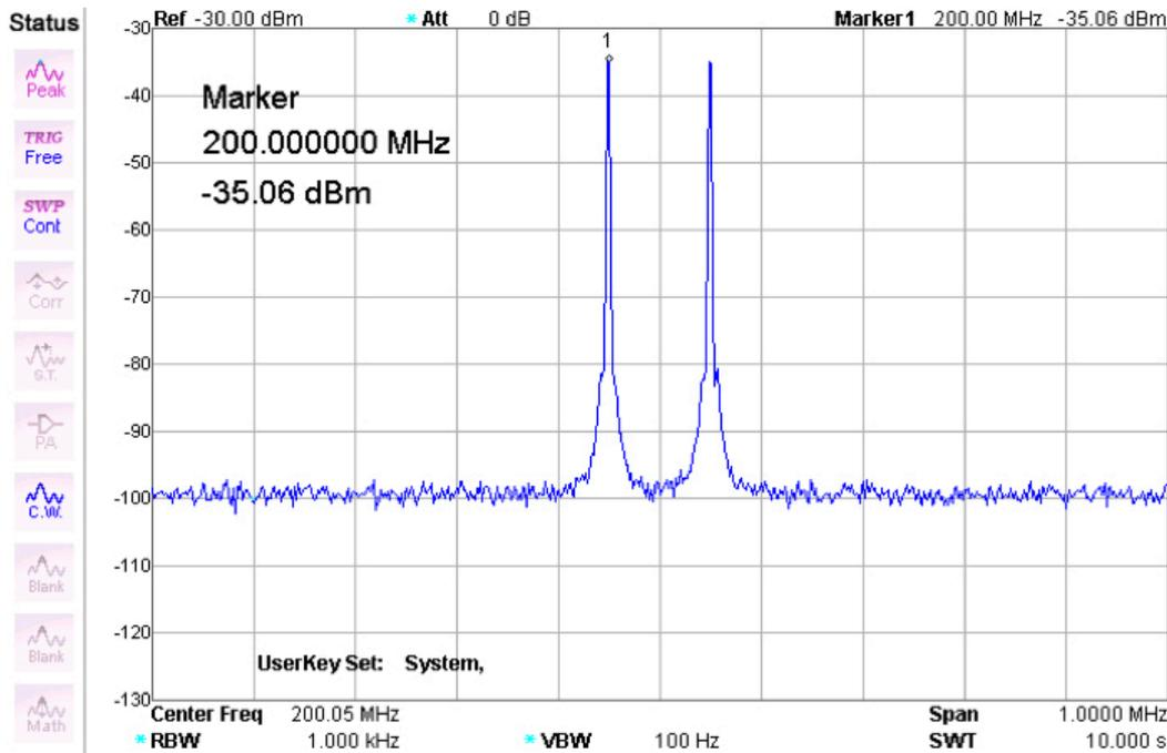
If there is no requirement to look at signals with amplitudes close to the noise floor, everything is fine. However, if the spectrum has to be checked for signals with amplitudes close to the noise floor of approximately -100 dBm, the internal pre-amplifier of the spectrum analyzer needs to be turned on.
