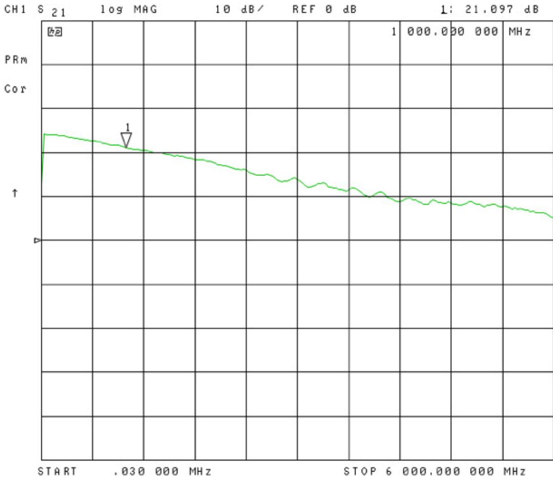
Picture 5 – TBHDR1, gain, 30 kHz – 6 GHz
