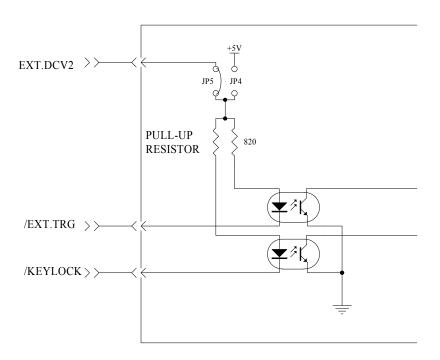
Figure 8 the input circuit for control signal
