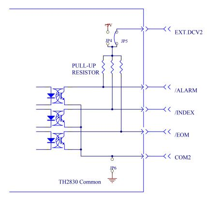
Figure 7 the output circuit for control signal
