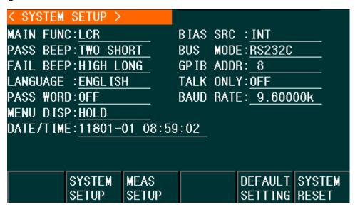
On this page, most system setup items are displayed, such as instrument main function, beeper, PASS beeper, FAIL beeper, language, PASS word, bus mode, GPIB address, TALK only, Bias SRC, baud rate, menu display and data/time.
