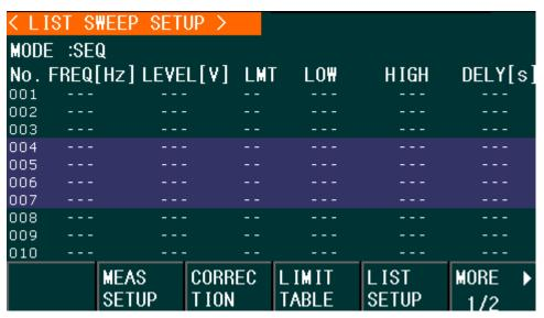
The list sweep function of TH2830 can perform auto sweep test for the test frequency, test level or bias voltage of 201 points. On **<LIST SWEEP SETUP>** page, the following list sweep parameters can be set.
