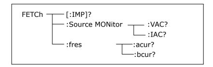
The FETCh[:IMP]? query directs TH2830 to input the last measurement result to the output buffer zone.
