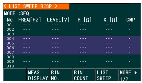
Test points will be automatically tested in a scanning mode. Meanwhile, comparison will be made between test results and limit values. In the process of list sweep test, "▶" denotes the current sweep test point. The following control parameters can be set on **<LIST SWEEP DISP>**.
