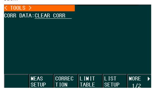
The TOOLS interface of TH2830 provides several specific functions and some custom design functions.
