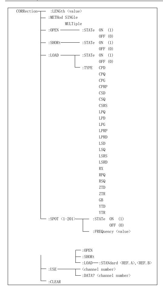
The CORRection: LENGth command is used to set the correction cable length. The
