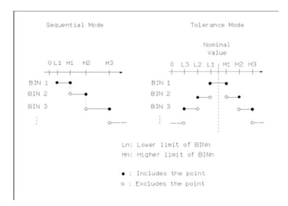
Figure 3-3 Tolerance mode and Sequential mode
