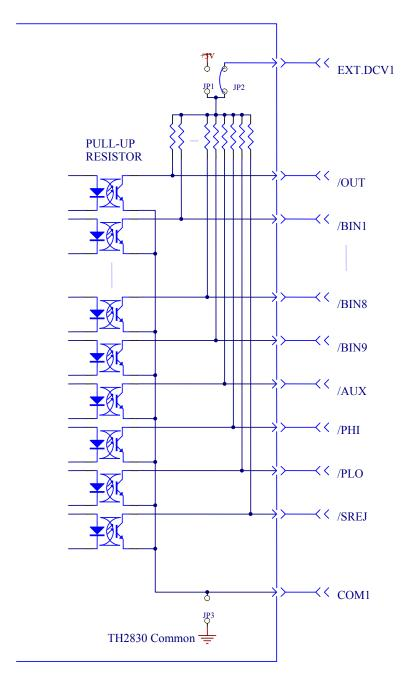
Figure 6 the output circuit for the comparison result
