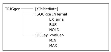
The TRIGger[:IMMediate] command is used to trigger a test.
