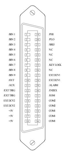
Note: the signal to /BIN1 - /BIN9, /OUT, /AUX, /PHI, /PLO and /SREJ in the list sweep comparison is different from that in the BIN comparison.
