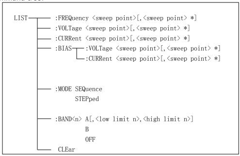
The LIST:FREQuency command is used to clear the original sweep points and set the frequencies of the sweep points. The LIST:FREQuency? query returns the current frequency of each sweep point.
