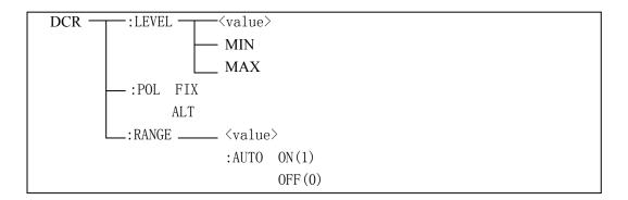
The DCR:LEVEL command is used to set the DCR level. The command DCR:LEVEL? query returns the current level.
