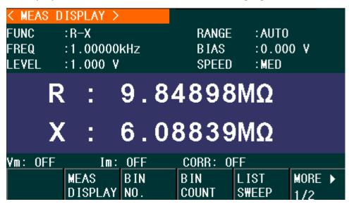
On this page, the test result is displayed in upper-case character. The measurement control parameters can be set on this page:
