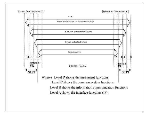
Figure 6-5 SCPI functions levels
