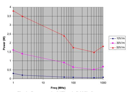
Fig. 4 Power required / Electric field Vs. frequency
