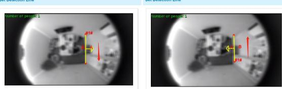
2) Ensure that the detected targets can pass through the detection line completely. It's recommended that the detection line is perpendicular to the In/Out direction and on the center of detection area without other objects around.
