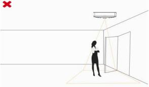
• Avoid installing the sensor near a mirror or avoid drawing the line to the mirror.
