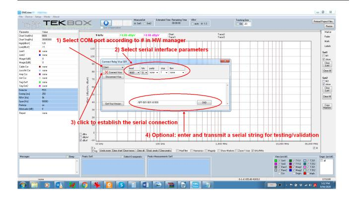
In order to automatically transmit test strings, they need to be entered into the desired segment file. You can add two serial command strings to each segment. Command SCPI\_A will be executed before the sweep of the corresponding segment. Command SCPI\_B will be executed after the sweep of the corresponding segment.
