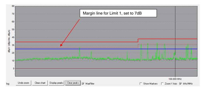
By default, the margins are set to 0, so any peak crossing the limit line would be indicated. Setting margin1 to e.g. 7dB would select all peaks coming within 7 dB close to the limit line of the graph measured with Settings1. Peaks crossing the margin line or limit line can be listed in the in the **Peaks window** by pressing the **Display peaks** button. See chapter 19 on how to manually select peaks and transfer it into the peaks list.
