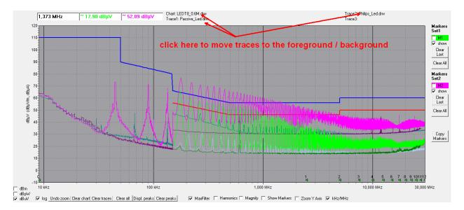
Charts are always saved including the amplitude correction data. If you figure out, that you applied wrong correction files, after completing a measurement, you can save the chart and then reload it as raw data and select different amplitude correction files.
