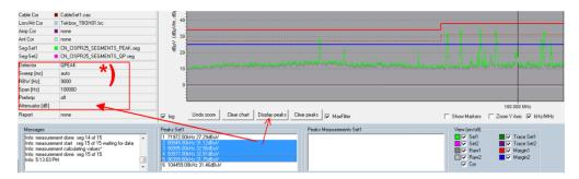
The software will then re-measure, using the selected peaks as center frequency and using the detector, sweep time, RBW, Span and PreAmp settings defined in the control box. This feature is a short cut to make a fast Quasi Peak measurement for selected peaks, instead of making a time consuming full span QP measurement.
