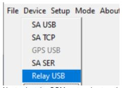
Next select the COM port and set up the parameters for the serial interface of the relay controller or any other serial device. Establish the connection and optionally transmit a string for testing/validation:
