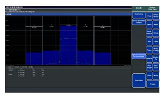
ACLR Test for 5G NR Base Station Signal (100 MHz BW)
