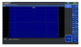
OBW Test for 5G NR Base Station Signal (100 MHz BW)
