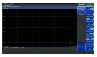
Channel Power Test for 5G NR Base Station Signal (100
